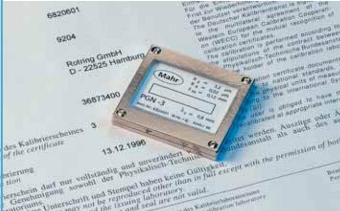
Surface roughness standard with a sinusoidal groove profile. Profile depth approx.  $3\ \mu\text{m}$  ( $120\ \mu\text{in}$ ), groove spacing approx.  $0.12\ \text{mm}$  ( $.00472\ \text{in}$ ). For checking the roughness measuring station. The following types are available:
