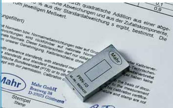
with Mahr calibration certificate. Roughness standard with turned profile, chromed. Profile depth approx.  $10\ \mu\text{m}$  ( $.394\ \mu\text{in}$ ). For checking the roughness measuring station.  $R_a$ ,  $R_z$ ,  $R_{\text{max}}$ .
