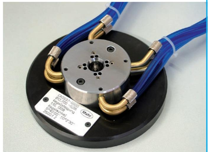
*Taper jet air ring gage with 2 measuring paths on 2 planes each to test 4x diameter, 2x taper angle, 2x taper pitch*
