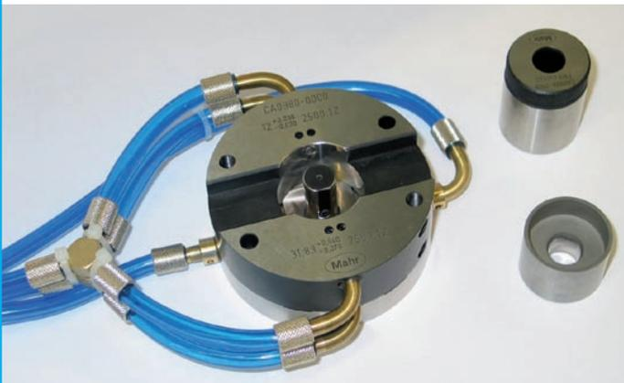
Pneumatic combination measuring device
