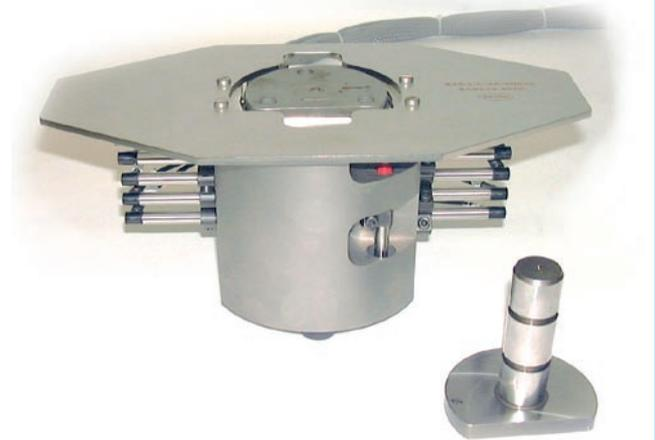
*Electronic multi-gage measuring device to test 6x diameter and perpendicularity*
