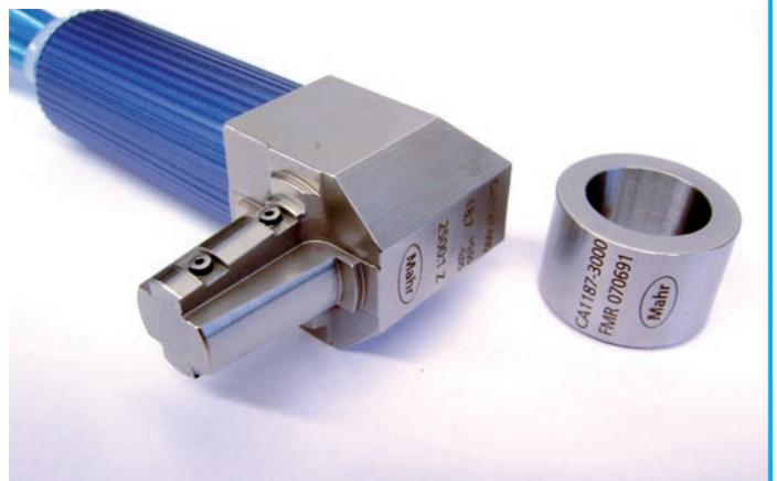
*Taper air plug gage with fixed attachment*
