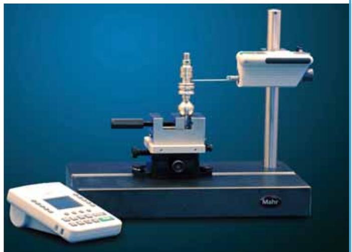
MarSurf measuring station with measuring stand ST-G
