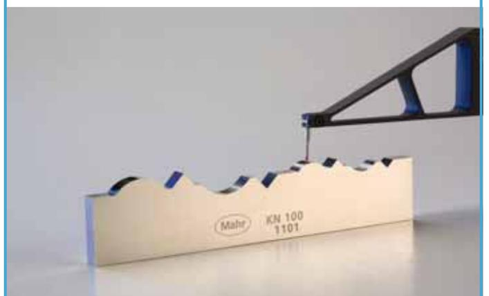
The contour standard **KN 100** was developed in cooperation with the PTB. Testing for confirmation and acceptance purposes can now be conducted traceable back to the PTB due to concrete reference to realistic geometries. The standard fulfills the requirements of the VDI/VDE guidelines 2629.
