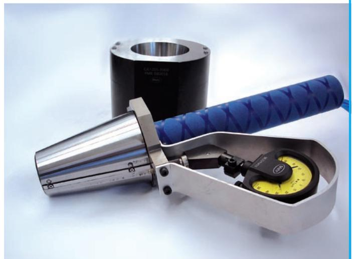
*Taper air plug gage with taper attachment*
