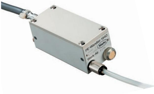
Air-controlled probes are becoming more and more widespread in dimensional metrology. Air / electronic converters convert the measuring signal (air pressure) into an electronic signal.
