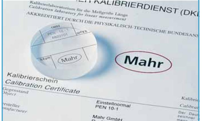
Depth setting standard for the static calibration of the vertical stroke of all skidless, single-skid and dual-skid probes. Groove depth approx.  $10\ \mu\text{m}$ ,  $\varnothing 44\ \text{mm}$ .
