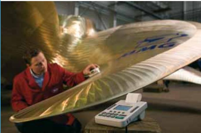
Roughness measurement on ship propellers (Mecklenburger Metallguss)
