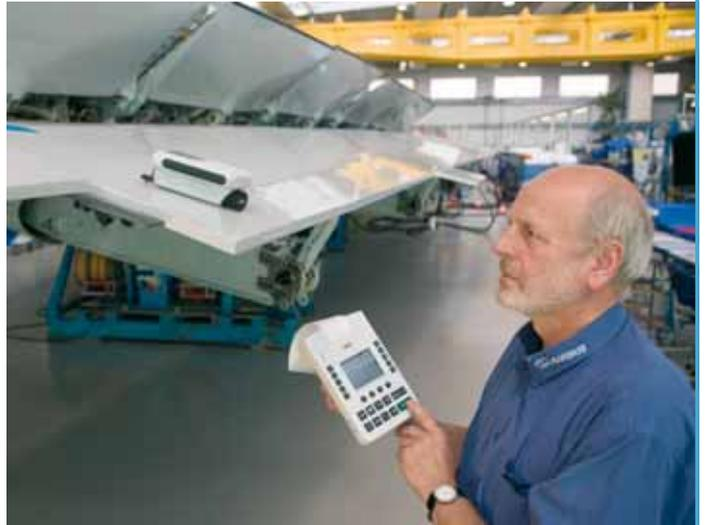
Roughness measurement on wings (Airbus)
